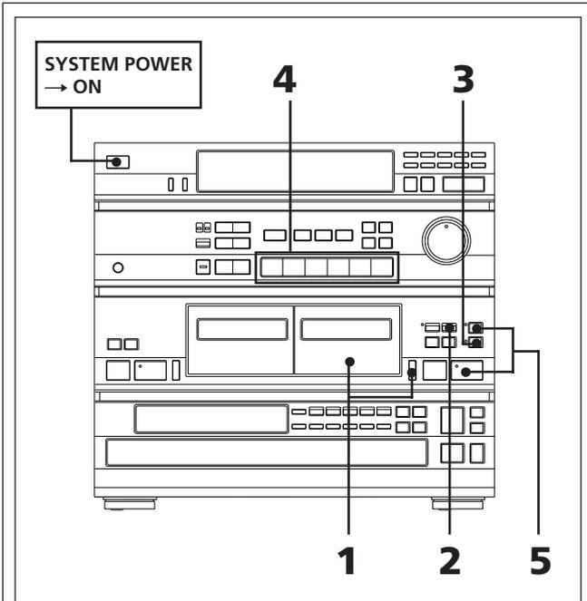
**1** Press to open the cassette compartment, insert the tape with the side to be recorded facing you and close the cassette compartment.
