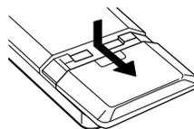
**2** Insert two size-AA (R6) batteries with correct polarity.
