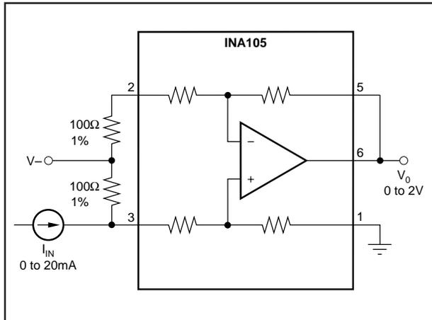
FIGURE 5. Current Receiver with Compliance to Rails.
