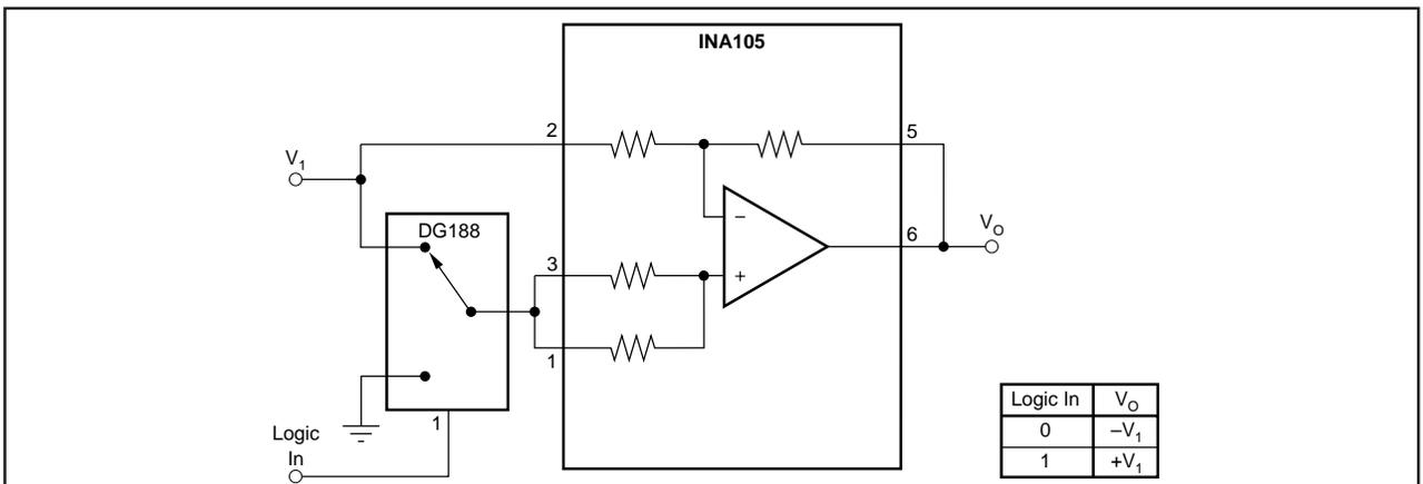
FIGURE 26. Digitally Controlled Gain of ±1 Amplifier.
