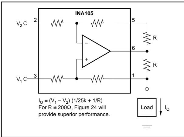
FIGURE 19. Precision Voltage-to-Current Converter with Differential Inputs.
