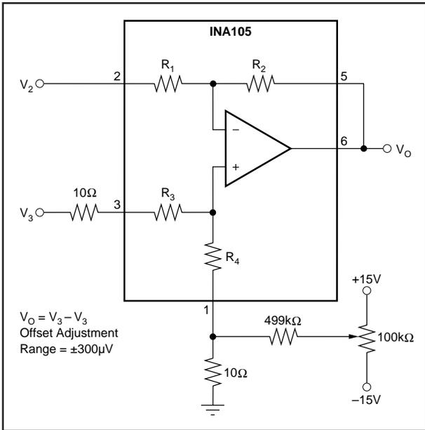
FIGURE 2. Offset Adjustment.
