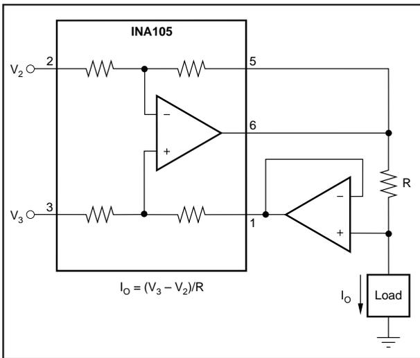
FIGURE 20. Differential Input Voltage-to-Current Converter for Low  $I_{OUT}$ .
