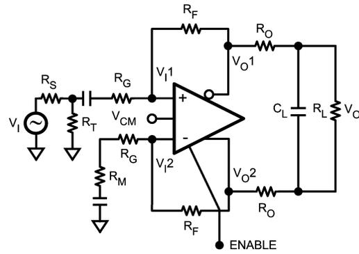
$$*V_{CM} = \frac{V_{O1} + V_{O2}}{2} \quad V_{ICM} = V_{OCM}$$
