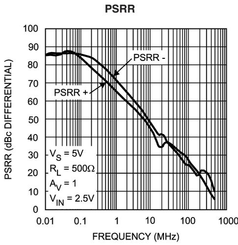
**Typical Performance Characteristics** ( $T_A = 25^\circ\text{C}$ ,  $V_S = \pm 5\text{V}$ ,  $R_L = 500\Omega$ ,  $R_F = 365\Omega$ ,  $A_V = +1$ ; Unless Specified). (Continued)
