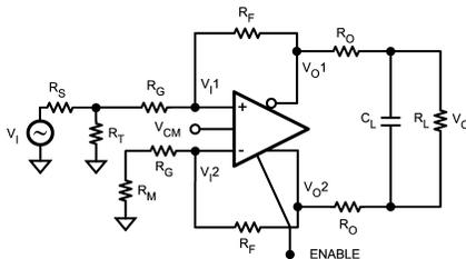
$$*V_{CM} = \frac{V_{O1} + V_{O2}}{2} \quad V_{ICM} = V_{OCM} * \frac{(R_G + R_M)}{(R_G + R_M + R_F)} \approx \frac{V_{OCM}}{1 + A_v} \quad \text{WHERE } R_M \ll R_G$$
