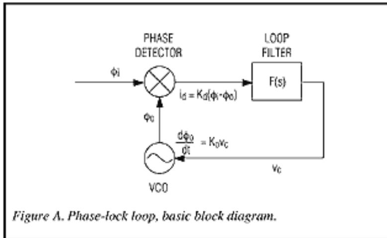
Figure A. Phase-lock loop, basic block diagram.
