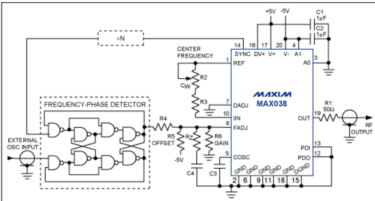
Figure 12. This discrete-gate frequency-phase detector allows use of an external  $\div N$  circuit, and assures that the PLL will lock only to the fundamental (not a harmonic) of the applied frequency.
