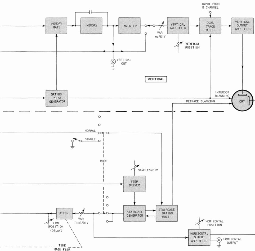
Fig. 2-3. Sequential-mode block diagram.
