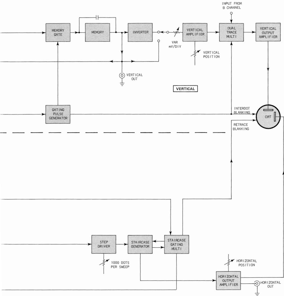
Fig. 2-9. Clocked real-time mode block diagram.
