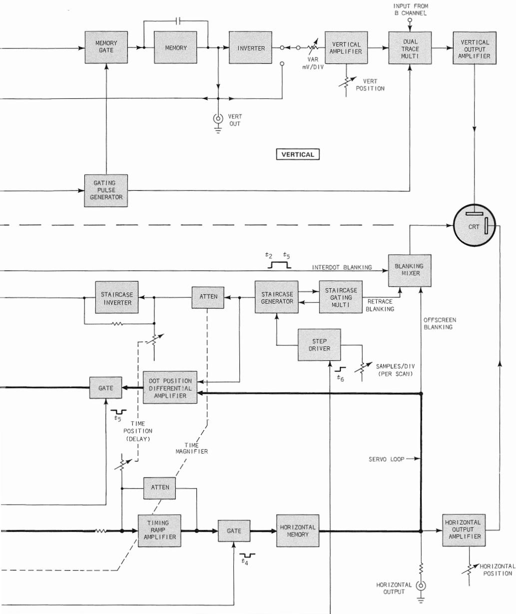
Fig. 2-6. Random-mode block diagram.
