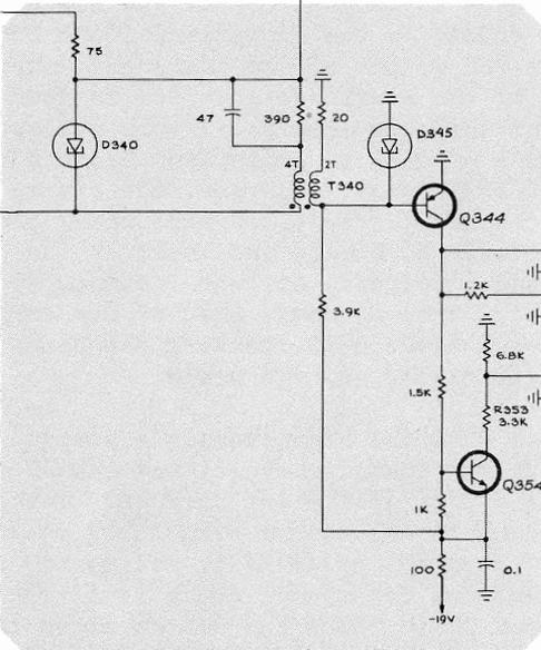
**FAST RAMP COMPARATOR AND SAMPLING COMMAND PULSE GENERATOR**
