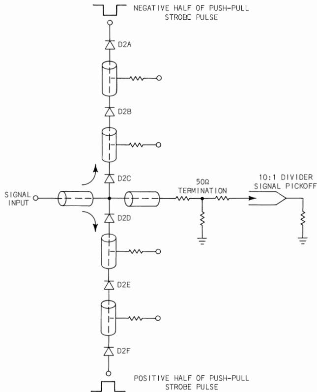
Fig. 3-13. Sampling-gate input.
