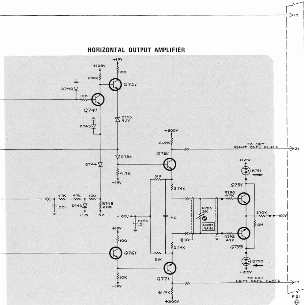
Fig. 6-3. 3T2 Horiz Amplifier and Blanking.
