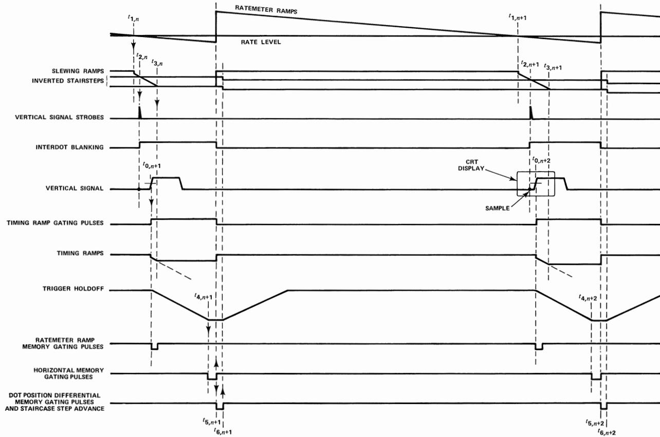
Fig. 2-7. Random-mode timing diagram.
