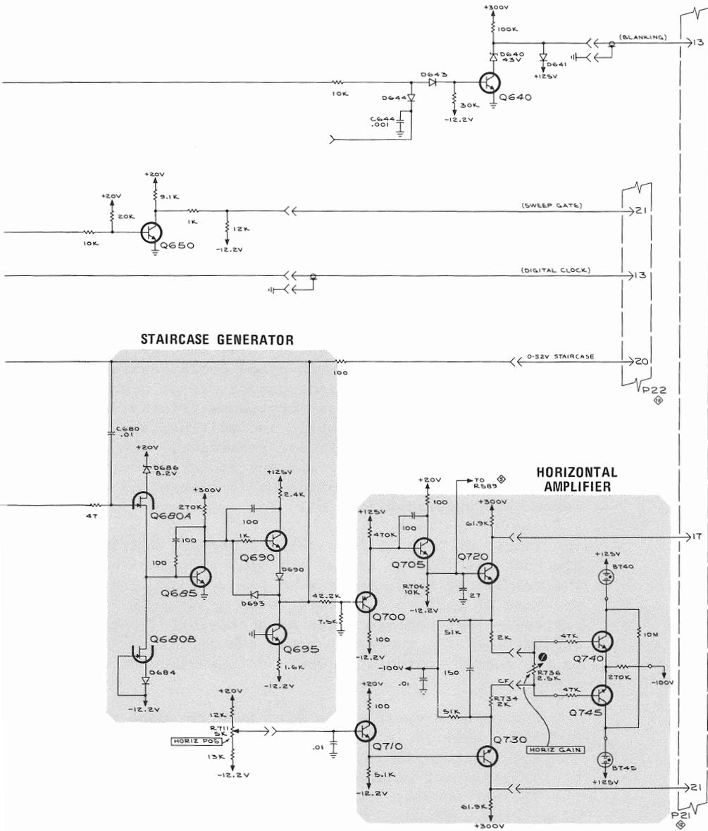
Fig. 5-7. 3T5 Staircase Gen and Horiz Amp.
