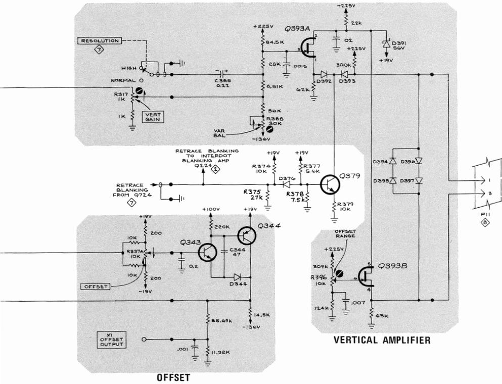
Fig. 3-3. 1S2 Offset and Output Stage.
