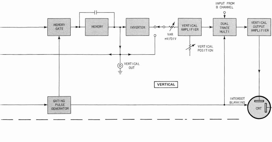
Fig. 2-1. Basic block diagram of vertical deflection section.
