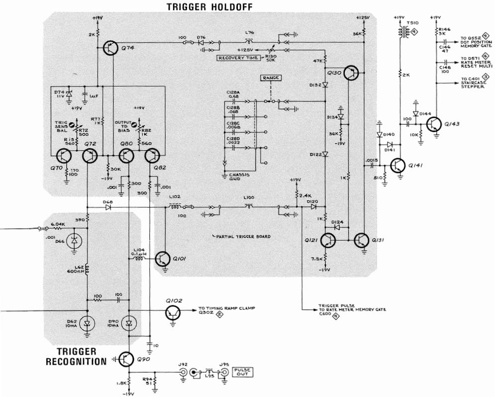
Fig. 4-5. 3T2 Trigger and Holdoff.
