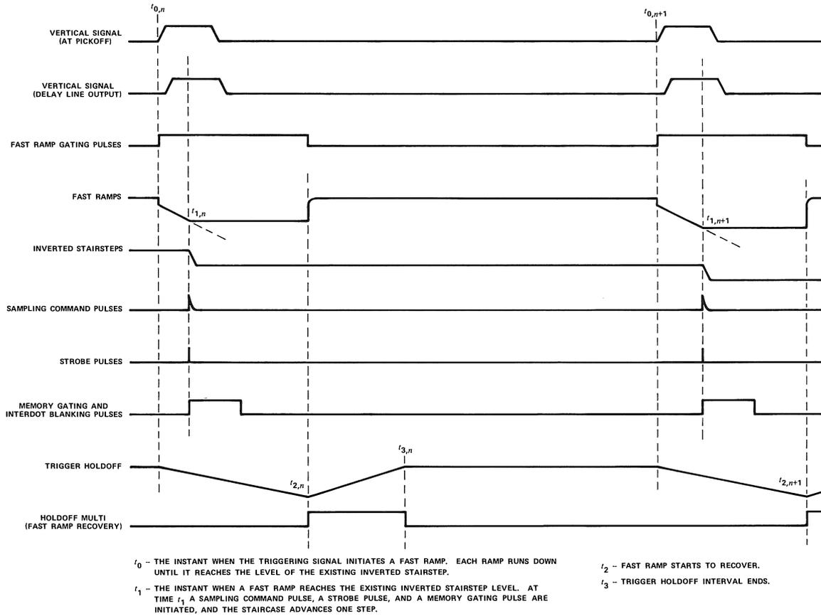
Fig. 2-4. Sequential-mode timing diagram.
