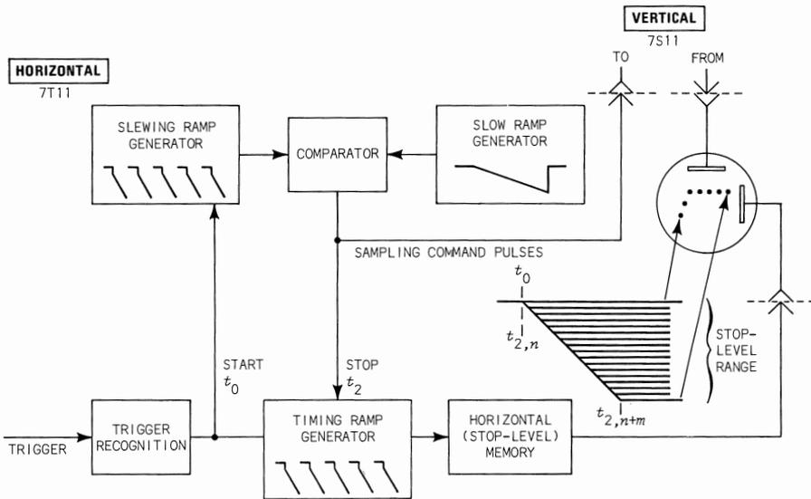
Fig. 2-5. 7T11 sequential mode (simplified).
