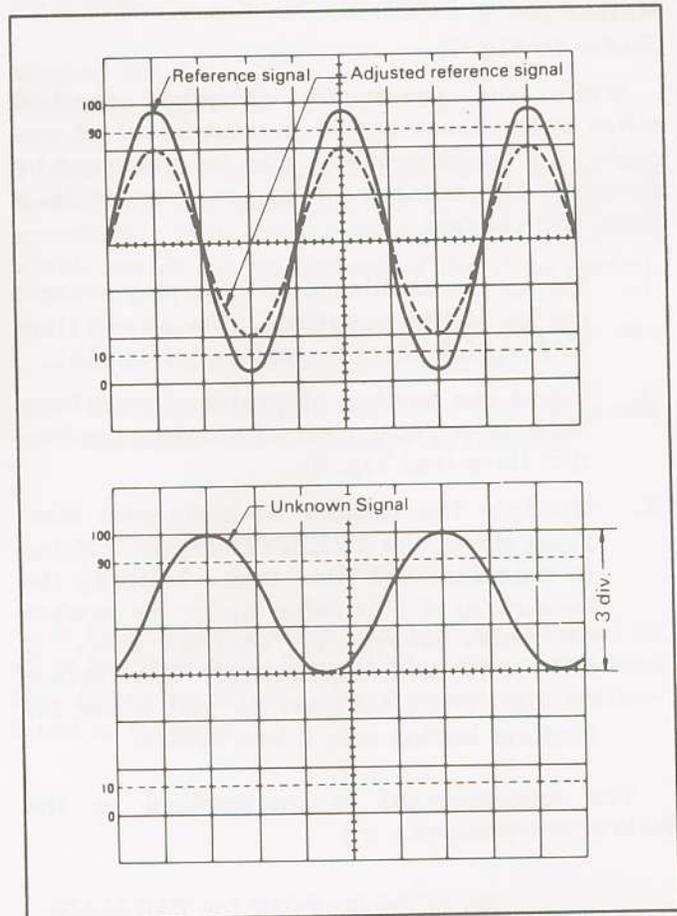
Fig. 11. Voltage Measurement, Relative Method.
