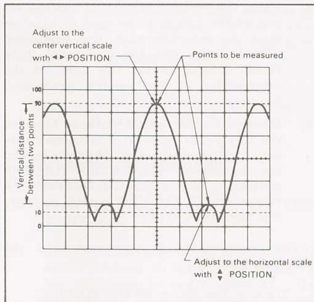
Fig. 6. Voltage Measurement.
