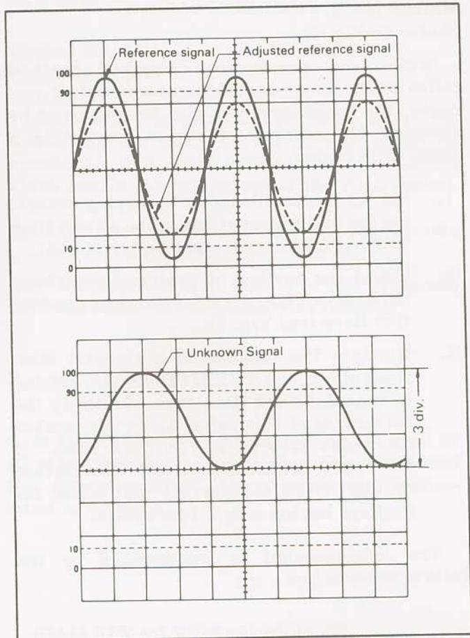
Fig. 11. Voltage Measurement, Relative Method.
