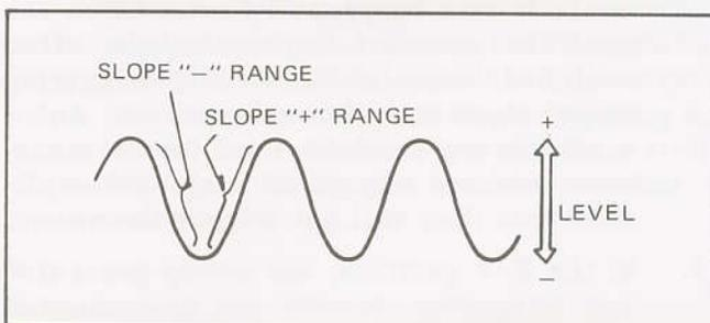
Fig. 4. Function of Slope and Level Controls.
