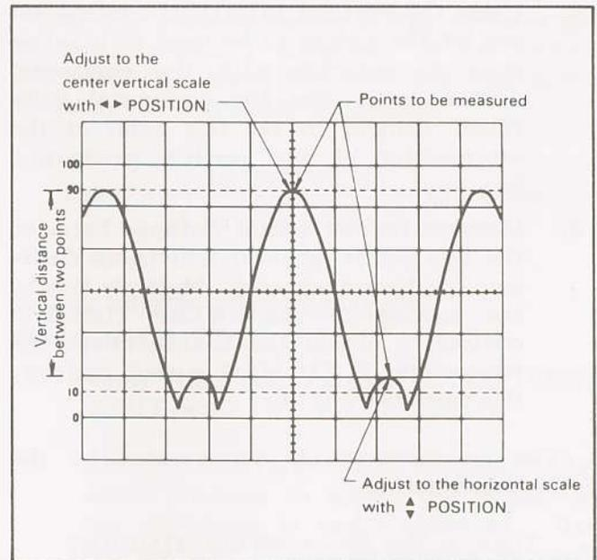
Fig. 6. Voltage Measurement.
