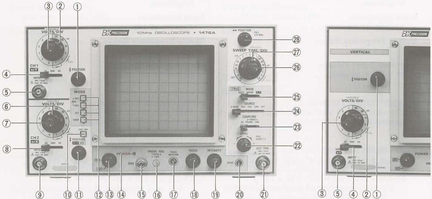
Fig. 1. Front Panel Controls and Indicators.
