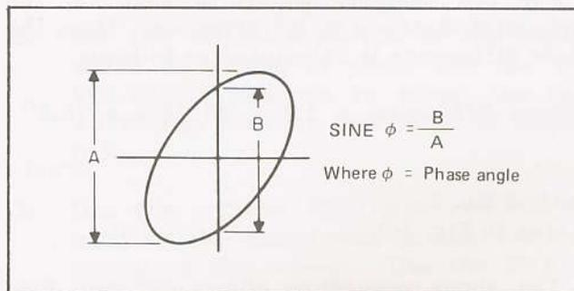
Fig. 18. Phase Measurement, X-Y Operation.
