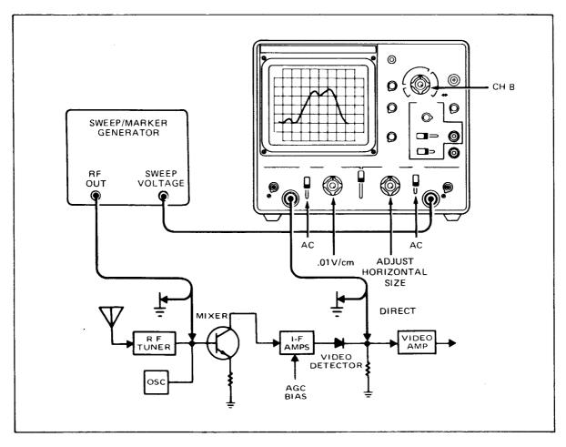
Fig. 29. Typical IF alignment set-up.
