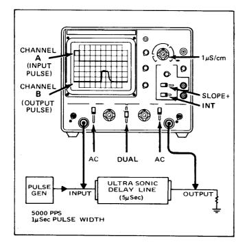
Fig. 12. Delay line measurement.
