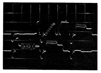
Fig. 15. Oscilloscope presentation of fields 1 and 2 of VITS information.
