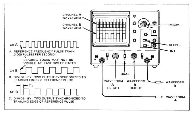
Fig. 7. Waveforms in divide-by-two circuit.
