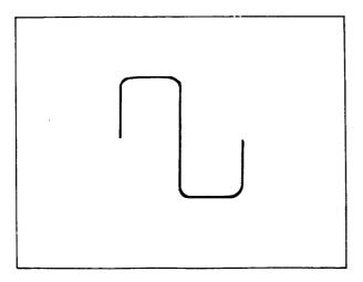
Fig. 39. Square wave response with high frequency loss.
