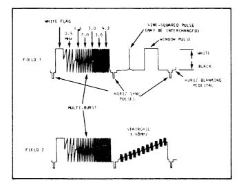
Fig. 20. Typical VITS signal, fields 1 and 2.
