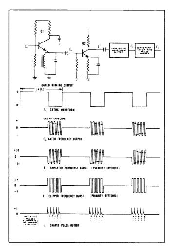
Fig. 11. Gated ringing circuit and waveform.
