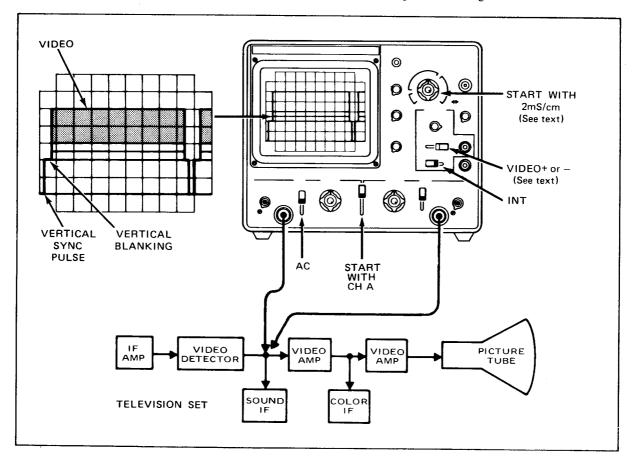
Fig. 17. Set-up for viewing vertical fields of composite video signal.
