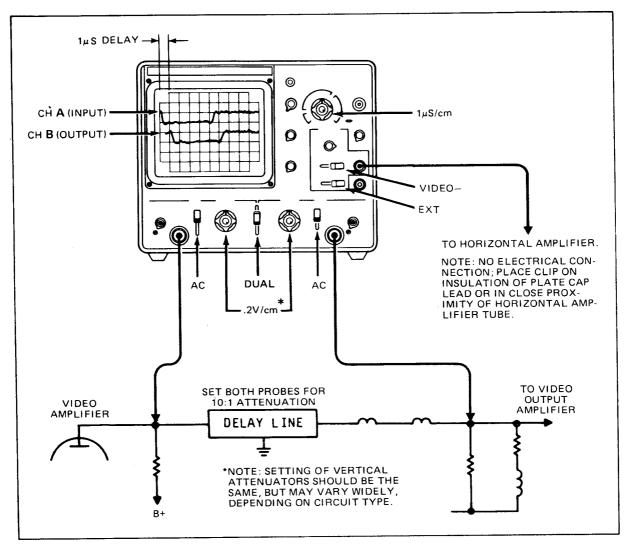
Fig. 13. Checking "Y" delay line in color television receivers.
