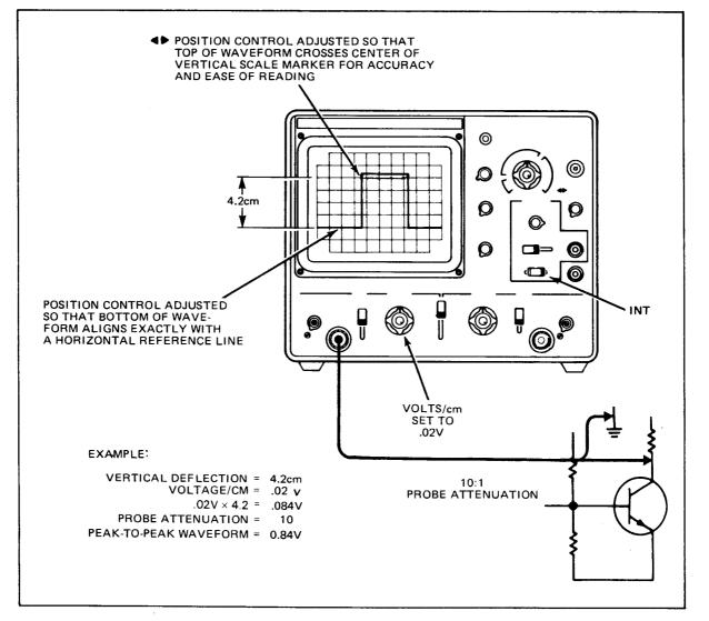
Fig. 4. Typical voltage measurement.
