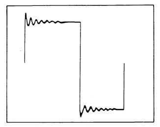
Fig. 47. Effect of high-frequency boost and poor damping.
