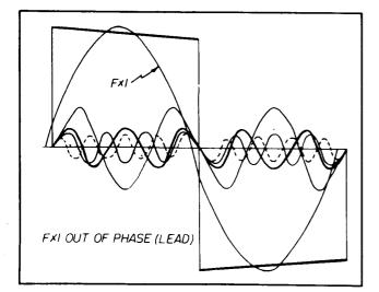
Fig. 44. Tilt resulting from phase shift of fundamental frequency in a leading direction.
