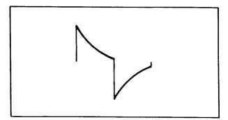
Fig. 46. Low-frequency component loss and phase shift.
