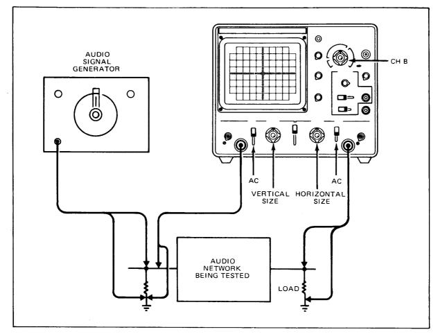
Fig. 34. Typical phase measurement alignment set-up.
