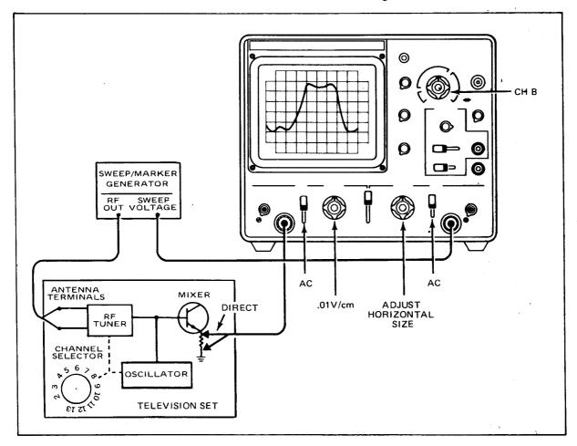
Fig. 28. Typical tuner alignment set-up.
