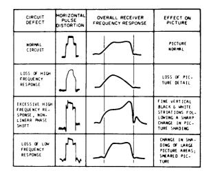
Fig. 18. Analysis of sync pulse distortion.
