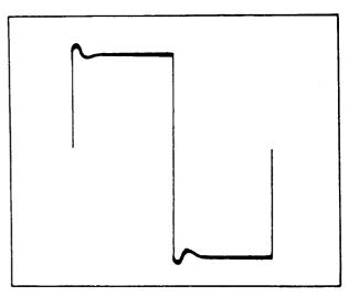
Fig. 48. Effect of high-frequency boost and good damping.
