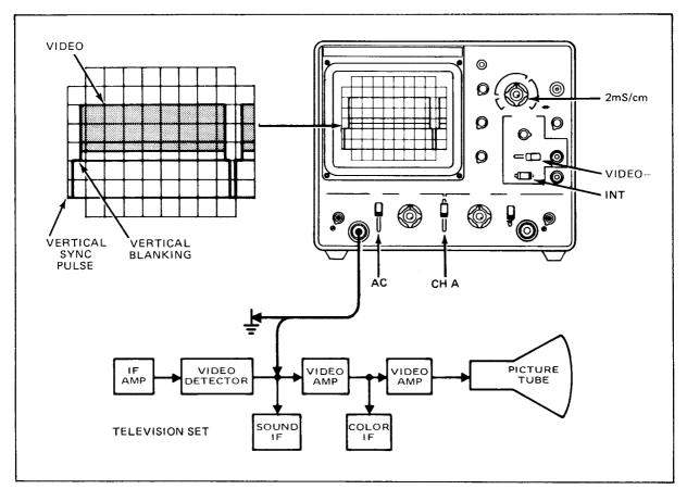
Fig. 14. Set-up for viewing fields 1 and 2 of VITS information.
