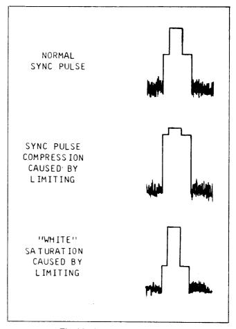
Fig. 19. Sync pulse waveforms.
