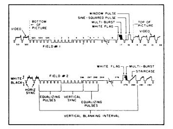
Fig. 21. Vertical blanking interval, showing typical VITS information.
