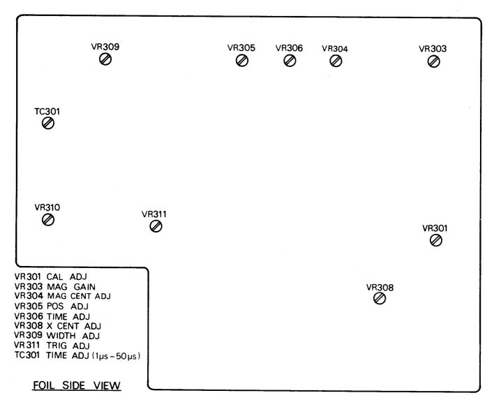
Fig. 52. Calibration diagram, horizontal amplifier board.
