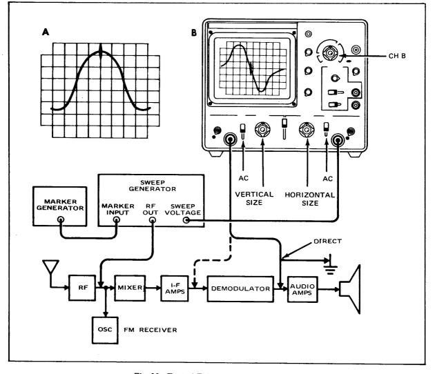
Fig. 33. Typical FM receiver alignment set-up.
