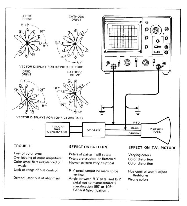
Fig. 26. Vectorscope operation and patterns.
