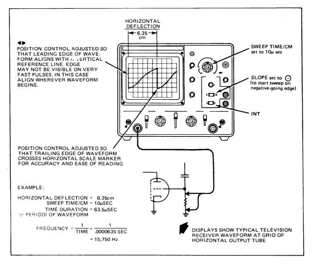
Fig. 5. Typical time measurement.
