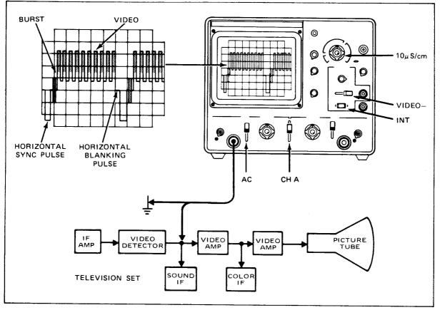
Fig. 16. Set-up for viewing horizontal lines of composite video signal.
