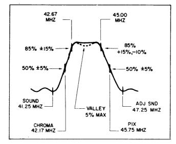
Fig. 30. Typical IF response curve, showing tolerance ranges of response levels.
