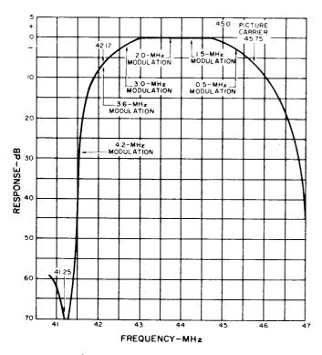
Fig. 23. Color TV IF amplifier response curve.
