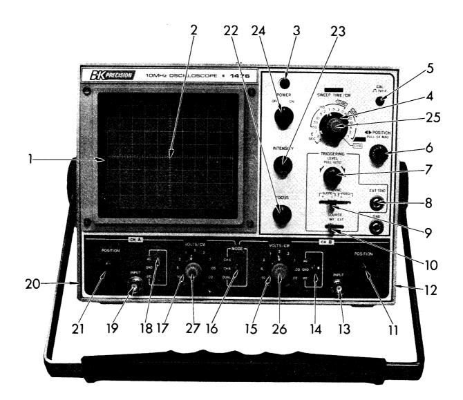
Fig. 1. Front panel controls and indicators.
