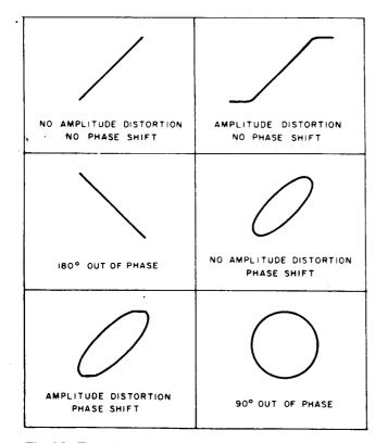
Fig. 35. Typical phase measurement oscilloscope displays.
