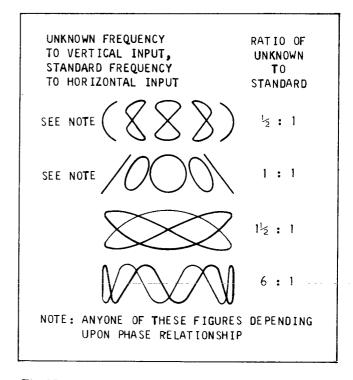
Fig. 37. Lissajous waveforms used for frequency measurement.
