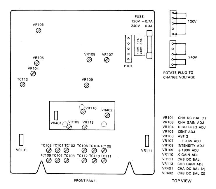
Fig. 51. Calibration diagram, vertical amplifier and power supply board.
