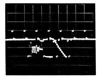
Fig. 22. Oscilloscope presentation of VITS information, single-trace operation.
