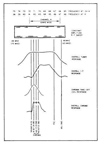
Fig. 27. TV response curves obtained by sweep-frequency technique.
