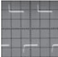
1MHz signal with improperly adjusted probe
