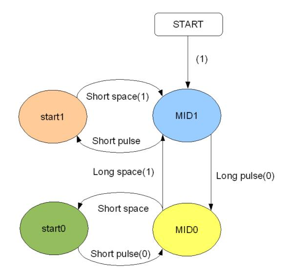
At 125 KHz, the bit time is 512 uS. A short pulse we define as halve a bit time which is 256 uS.
