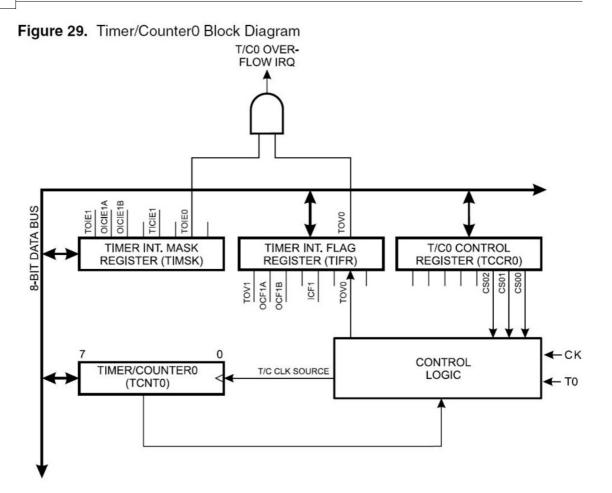
The 8-bit Timer/Counter0 features both a high resolution and a high accuracy mode with lower pre-scaling values. Similarly, high pre-scaling values make the Timer/ Counter0 useful for lower speed functions or exact timing functions with infrequent actions.
