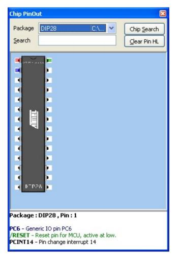
When you move the mouse cursor over a pin, you will see that the pin will be colored red. At the bottom of the window, a pin description is show. In the sample above you will see that each line has a different color. This means that the pin has multiple alternative functions.
