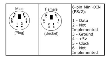
Old PC's are equipped with a 5-pin DIN female connector. Newer PC's have a 6-pin mini DIN female connector.
