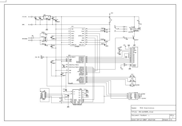
As you can see from the data sheets, the EM4095 needs little external hardware. A coil, capacitors that tune the coil for 125 KHz, are basically all that you need. IC1 is a voltage regulator that regulates the input voltage to 5V. (you can operate it from a 9V battery). The capacitors stabilize the output voltage. The DEMOD output of the EM4095 is connected to the microprocessor and the pin is used in input mode. The MOD and SHD pins are connected to micro pins that are used in output mode.
