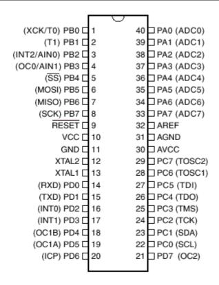
The JTAG interface is enabled by default. This means that portC.2-portC.5 pins can not be used. Program the JTAG fuse bit to disable the JTAG interface.
