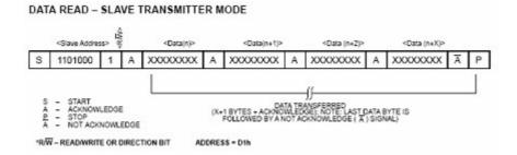
Again the start condition and the slave address, only this time the master sends "1" for the R/W bit. The slave can then begin to send after the acknowledge. If the master wishes to stop receiving it should send a not acknowledge.
