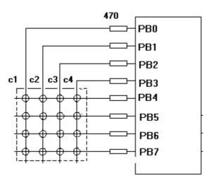
Note that the port pins can be used for other tasks as well. But you might need to set the port direction of those pins after you have used getkbd(). For example the LCD pins are set to output at the start of your program. A call to getkbd() would set the pins to input.
