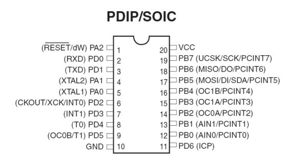
The tiny4313 has an internal oscillator that can run at various frequencies. The 4 MHz seems not to work precise. when using the UART for serial communication you can get wrong output. You can best use the 8 MHz internal oscillator , or tweak the UBRR register. For example, UBRR=UBRR+1 That worked for 4 Mhz, at 19200 baud.
