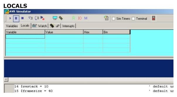
The LOCALS window shows the variables found in a SUB or FUNCTION. Only local variables are shown. You can not add variables in the LOCALS section. Changing the value of local variables works the same as in the Variables TAB.
