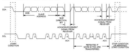
As said a data transfer can occur after a **start condition** of the master. The length of data sent over I<sup>2</sup>C is always 8 bit this includes a read/write direction bit, so you can effectively send 7 bits every time.
