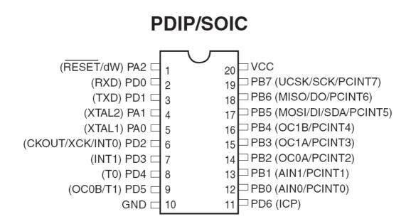
The tiny2313 has an internal oscillator that can run at various frequencies. The 4 MHz seems not to work precise. when using the UART for serial communication you can get wrong output. You can best use the 8 MHz internal oscillator , or tweak the UBRR register. For example, UBRR=UBRR+1 That worked for 4 Mhz, at 19200 baud.
