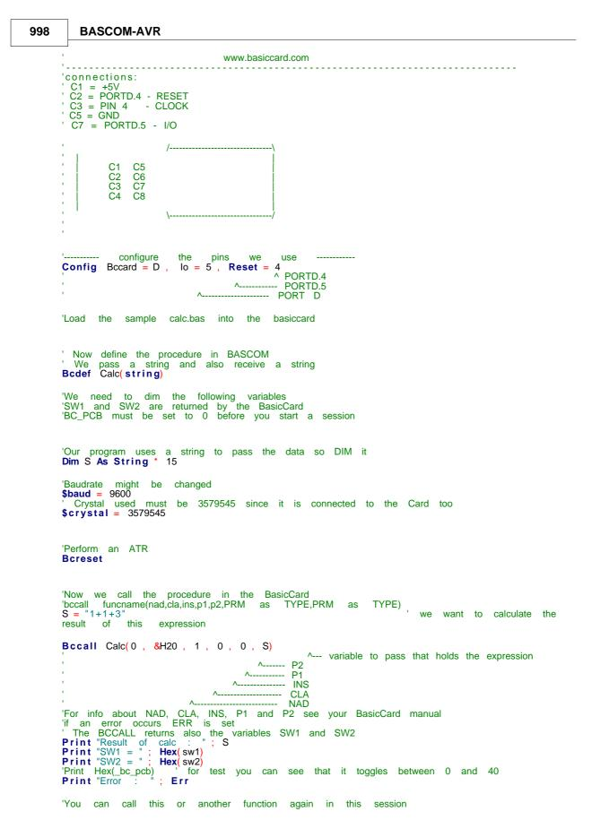
$\begin{array}{l} S = "2+2"\\ \textbf{Bccall Calc}(0, \& H20, 1, 0, 0, S)\\ \textbf{Print "Result of calc : "; S}\\ \textbf{Print "SW1 = "; Hex(sw1)}\\ \textbf{Print "SW2 = "; Hex(sw2)}\\ \textbf{'Print Hex(\_bc\_pcb)} & \text{for test you can see that it toggles between 0 and 40} \end{array}$
