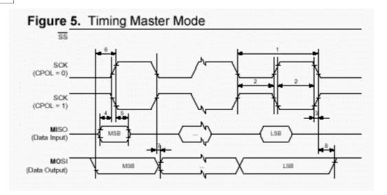
The minimum timing of the clock signal is given by the times "1" and "2". The value "1" specifies the SCK period while the value "2" specifies the high / low times of the clock signal. The maximum rise and fall time of the SCK signal is specified by the time "3". These are the first timings of the AVR to check if they match the requirements of the slave.
