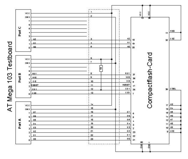
A typical connection to the micro is shown below.
