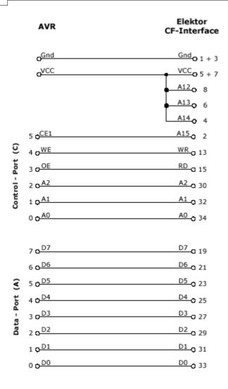
Changes of the hardware pins is possible in the file Config\_FlashCardDrive\_EL\_PIN. bas.
