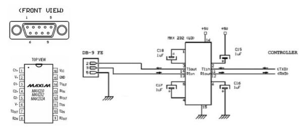
The DB-9 connector has 9 pins but you only need to use 3 of them. Notice that the drawing above shows the FRONT VIEW thus remember that you are soldering on the other side. On most connectors the pin outs can also be found on the connector itself.
