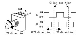
Since the microprocessor has internal pull up resistors, you do not need external pull up resistors for most encoders.
