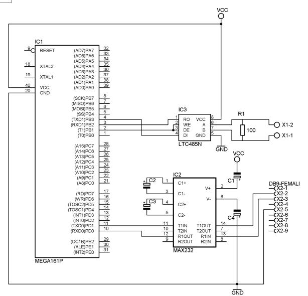
The sample above uses a MEGA161 or MEGA162 which has 2 UARTS. This way you can have both a RS232 and RS485 interface.
