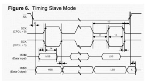
In principle the timings are the same in slave mode like previously described in master mode. Because of the switching of the roles between master and slave the requirements on the timing are inverted as well. The minimum times of the master mode are now maximum times and vice versa.
