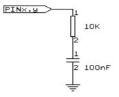
The capacitor is charged and the time it takes to discharge it is measured and stored in the variable. Now when you vary either the resistor or the capacitor, different values will be returned. This function is intended to return a relative position of a resistor wiper, not to return the value of the resistor. But with some calculations it can be retrieved.
