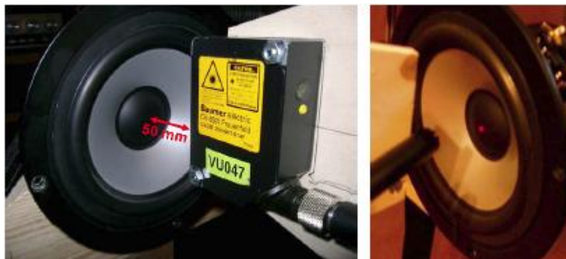
Figure 3.7. Positioning of laser displacement sensor and microphone
