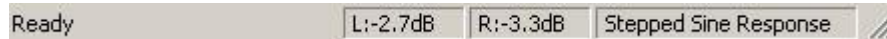
Figure 2.3 Status bar shows peak level (ref. full scale) of left and right line inputs
