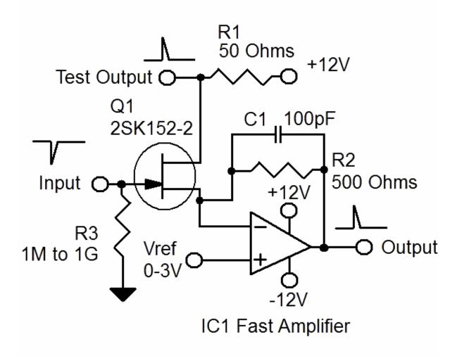
Figure 2 Very wide temperature range, gain-stable, fast JFET high-impedance amplifier
