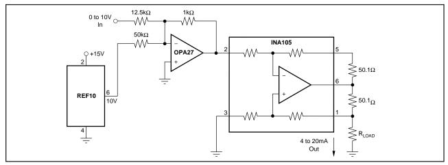
FIGURE 29. Precision 4-20mA Current Transmitter.
