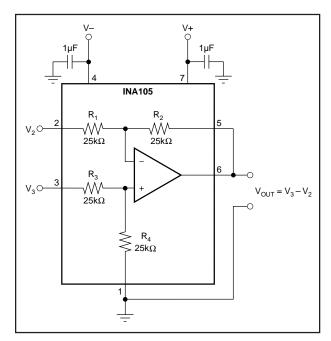
FIGURE 1. Basic Power Supply and Signal Connections.
