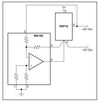
FIGURE 8. ±5V Precision Voltage Reference.
