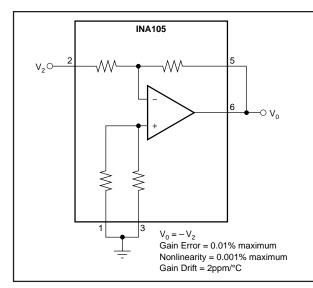
FIGURE 6. Precision Unity-Gain Inverting Amplifier.
