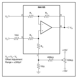
FIGURE 2. Offset Adjustment.
