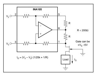
FIGURE 21. Isolating Current Source.
