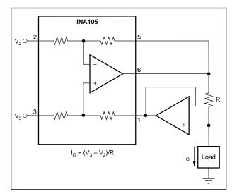
FIGURE 20. Differential Input Voltage-to-Current Converter for Low  $I_{OUT}$ .
