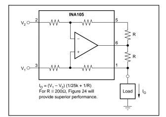
FIGURE 19. Precision Voltage-to-Current Converter with Differential Inputs.
