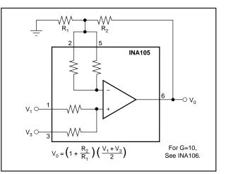
FIGURE 16. Precision Summing Amplifier with Gain.
