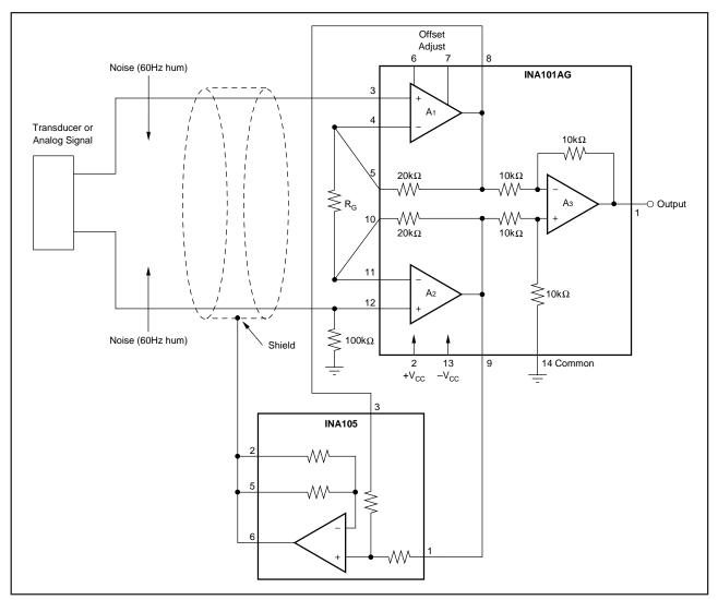
FIGURE 17. Instrumentation Amplifier Guard Drive Generator.
