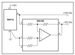
FIGURE 7. ±10V Precision Voltage Reference.
