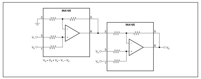
FIGURE 18. Precision Summing Instrumentation Amplifier.
