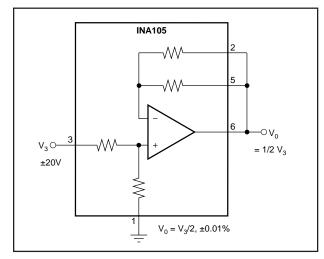
FIGURE 14. Precision Gain = 1/2 Amplifier.
