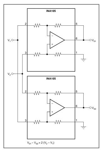
FIGURE 22. Differential Output Difference Amplifier.
