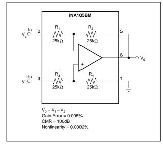
FIGURE 3. Precision Difference Amplifier.
