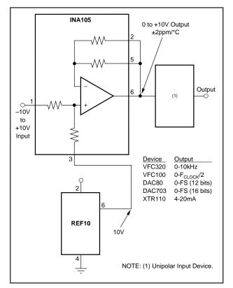
FIGURE 15. Precision Bipolar Offsetting.
