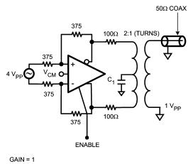
$C_1$  IS NOT REQUIRED IF  $V_{CM}$  = GROUND
