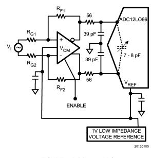
FIGURE 8. Driving an ADC
