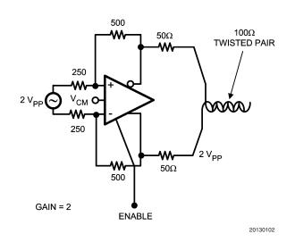
FIGURE 2. Fully Differential Cable Driver
