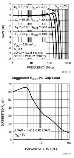
**Typical Performance Characteristics** ( $T_A = 25^{\circ}C$ ,  $V_S = \pm 5V$ ,  $R_L = 500\Omega$ ,  $R_F = 365\Omega$ ,  $A_V=+1$ ; Unless Specified). (Continued)
