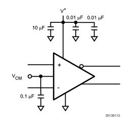
FIGURE 5. Single Supply Bypassing Capacitors
