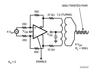
FIGURE 9. Transformer Out High Impedance Load
