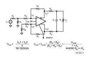
FIGURE 6. Relating Avto Input/Output Common Mode Voltages
