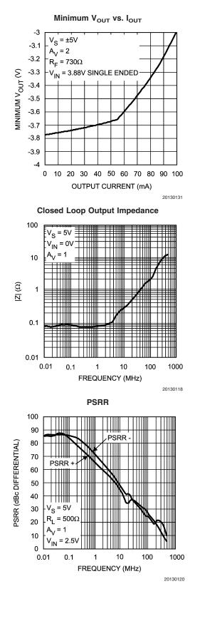
**Typical Performance Characteristics** ( $T_A = 25^{\circ}C$ ,  $V_S = \pm 5V$ ,  $R_L = 500\Omega$ ,  $R_F = 365\Omega$ ,  $A_V=+1$ ; Unless Specified). (Continued)
