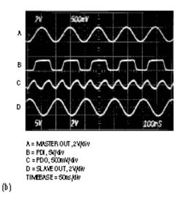
Figure 10. The SYNC output lets you synchronize one MAX038 to another.
