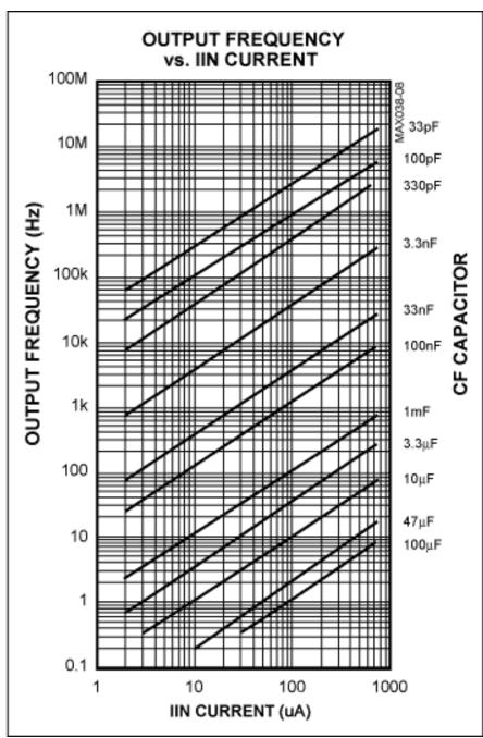
Figure 3. The output frequency in Figure 2 varies with current into IIN and the value of C<sub>F</sub>.
