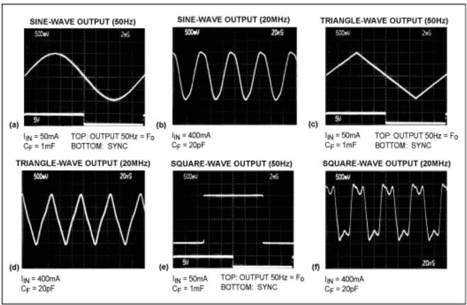
Figure 1. Among waveforms available at the MAX038 output are the sine (a, b), triangle (c, d), and square (e, f).
