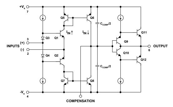
Figure 3: AD846 Current Feedback Op Amp (1988)
