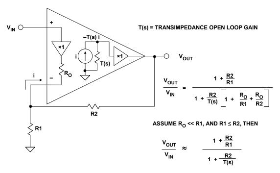
Figure 2: Current Feedback (CFB) Op Amp Topology
