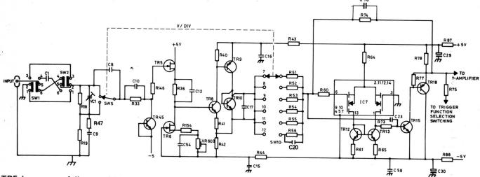
TR5 is a source follower with temperature compensation provided by current source TR6, which is I<sub>DSS</sub> matched with TR5. VR603, the rear panel DC offset control, adjusts the current source and therefore the DC level of TR8 base.
