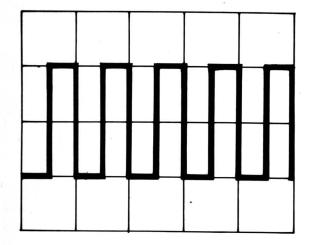
Adjust X-SHIFT so that trace starts at right hand side of the screen. Adjust VC2 for 1 cycle in 1 division at the left hand end of the trace.
