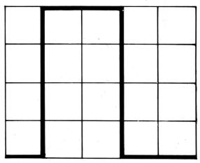
Readjust VR9 for a trace height of 4 divisions if necessary. Switch the TIME/DIV switch through all the ranges round to 500 and check that there is a linear progression in the change of the waveform displayed.
