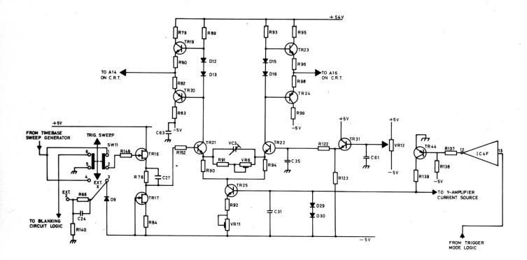
The ramp voltage from the timebase sweep generator is connected to the input of the X-amplifier when SW11 is in the TRIG SWEEP position.
