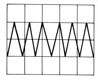
Adjust VC3 for best linearity (i.e. most even spaces between peaks). Adjust VR11 for maximum trace width at left hand end of the trace.
