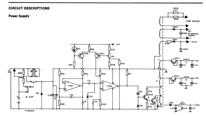
The power-supply is of the switched-mode type with regulation achieved by pulse-width modulation.
