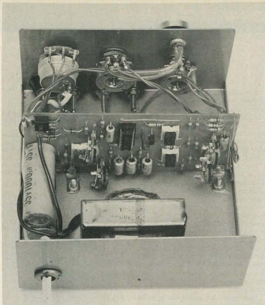
**INTERIOR VIEW** of fully-assembled unit showing details of point-to-point wiring. Angle brackets should contact bare metal in cabinet to assure good ground for shielding purposes. Binding posts are located just beneath front panel controls.
