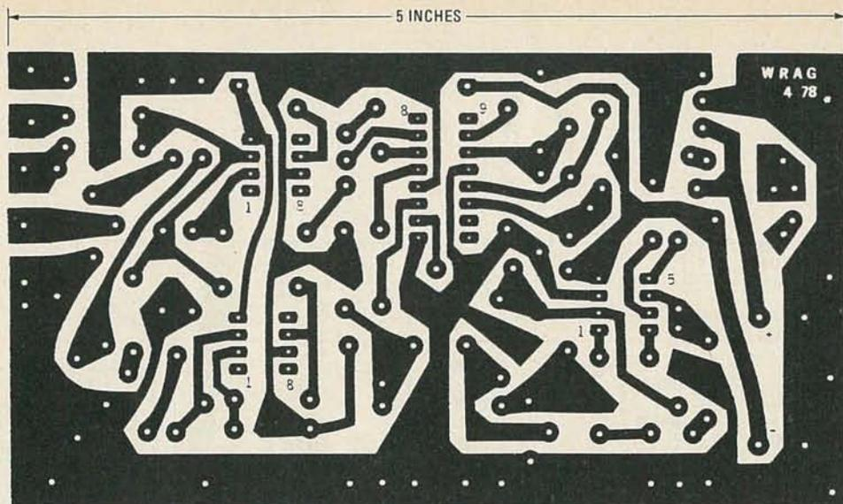
FIG. 3—FULL-SCALE reproduction of foil pattern of the Wide Range Audio Generator for those wishing to use PC board. Since parts placement is not critical, perforated board may also be used.
