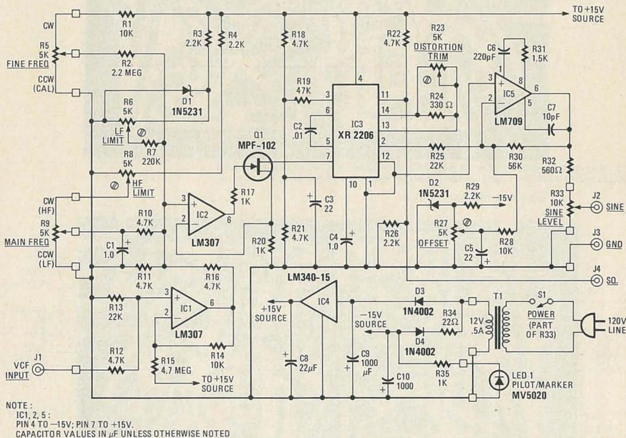
FIG. 2—FULL SCHEMATIC of the Wide Range Audio Generator. Power supply appears at lower right. VCF input (J1) permits external control of output frequency.
