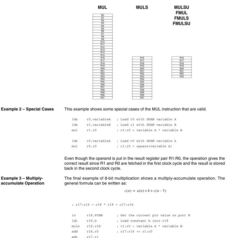
Typical applications for the multiply-accumulate operation are FIR (Finite Impulse Response) and IIR (Infinite Impulse Response) filters, PID regulators and FFT (Fast Fourier Transform). For these applications the FMULS instruction is particularly useful.
