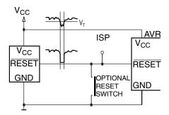
Figure 12. Integrated Reset Circuit with Adjustable Threshold Voltage
