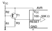
Figure 4. Low-cost Brown-out Detector with Manual Reset Button
