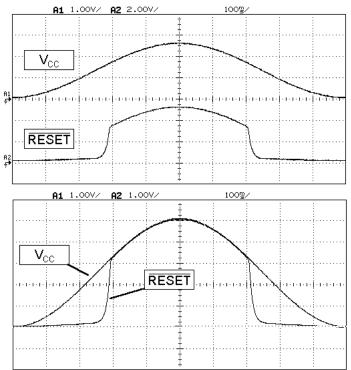
Figure 5. These Oscilloscope Plots Show how the Voltage on RESET Varies with  $V_{CC}$
