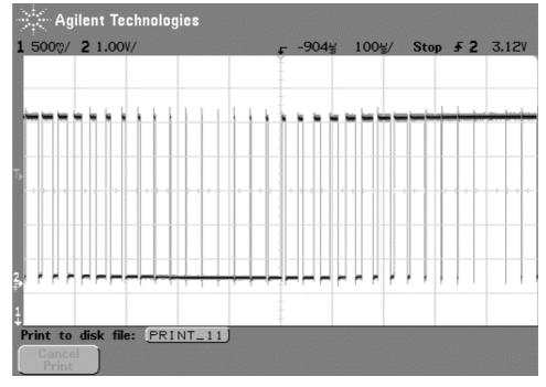
Figure 2. PWM Output with Varying Duty Cycle
