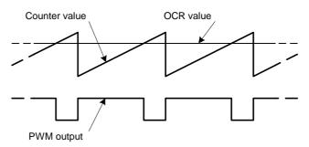
If using the high-speed PWM to generate analog signals, the step-size between the analog levels is depending on the resolution of the PWM. The higher base frequency the more easily is it to attenuate the base frequency and thereby minimize the signal ripple. The selection of resolution versus base frequency is thus an application dependent trade-off.
