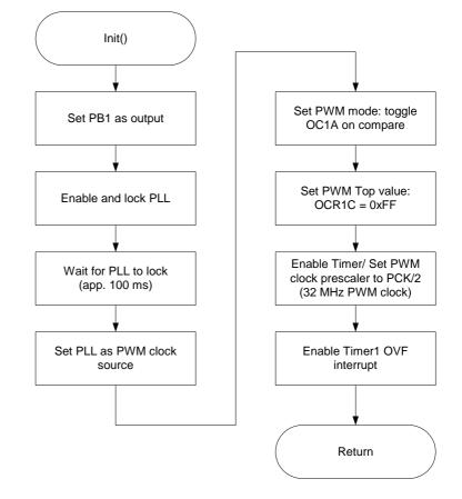
Figure 6. Init Routine, Initializes Pin and Timer1 to Operate in Fast PWM Mode
