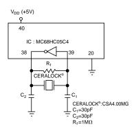
By actually setting up this circuit as well as the standard test circuit shown in Fig. 7-2, it is possible to establish the average shift that can be expected when using the CSA4.00MG with a 6805 processor. The actual data is shown below:
