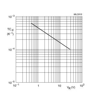
Fig.4 Temperature coefficient of diode capacitance as a function of reverse voltage; typical values.
