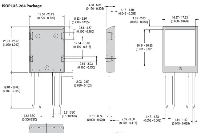
NOTE: Bottom heat sink meets  $2500V_{\rm rms}$  isolation to the pins.
