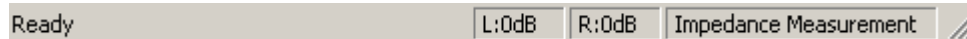
Figure 4.3 Status bar shows the peak level (ref. full scale) of left and right line inputs
