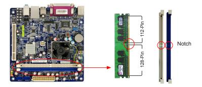
If you take a look at front side of memory module, it has asymmetric pin counts on both sides separated by a notch in the middle, so it can only fit in one direction. Follow the steps below to correctly install your memory modules into the sockets.
